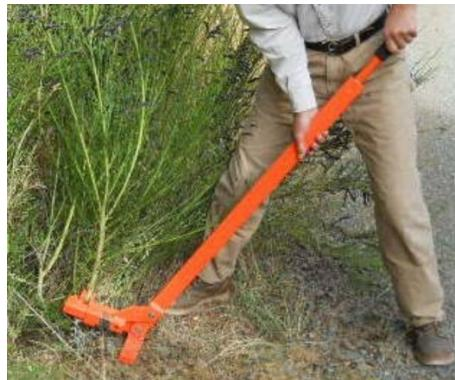
**Lopping Shears:** Used for cutting small buckthorn. Available for free with a \$25.00 deposit.
